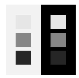
called *simultaneous contrast* causes the reproduced image to appear lacking in contrast, as demonstrated above. The effect can be overcome by applying an end-to-end power function whose exponent is about 1.1 or 1.2. Rather than having each receiver provide this correction, the assumed 2.5-power at the CRT is under-corrected at the camera by using an exponent of about  $\frac{1}{2.2}$  instead of  $\frac{1}{2.5}$ . The assumption of a dim viewing environment is built into video coding.
