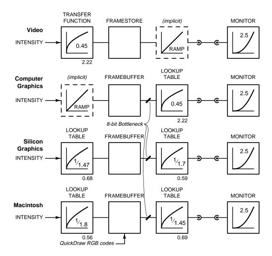
Synthetic computer graphics calculates the interaction of light and objects. These interactions are in the physical domain, and must be calculated in linear-light values. It is conventional in computer graphics to store linear-light values in the framebuffer, and introduce gamma correction at the lookup table at the output of the framebuffer. This is illustrated in the second row.
